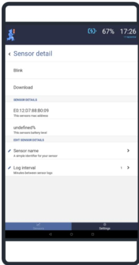
**Blink:** Pressing here will cause the sensor light to flash. You can use this feature to ensure that you are working with the correct sensor.
