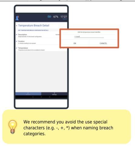
**Duration:** Using the slider, you can determine how long the temperature must continuously remain outside of the required temperature range for it to be considered a breach. You can set the duration to any length between 1 and 600 minutes.
