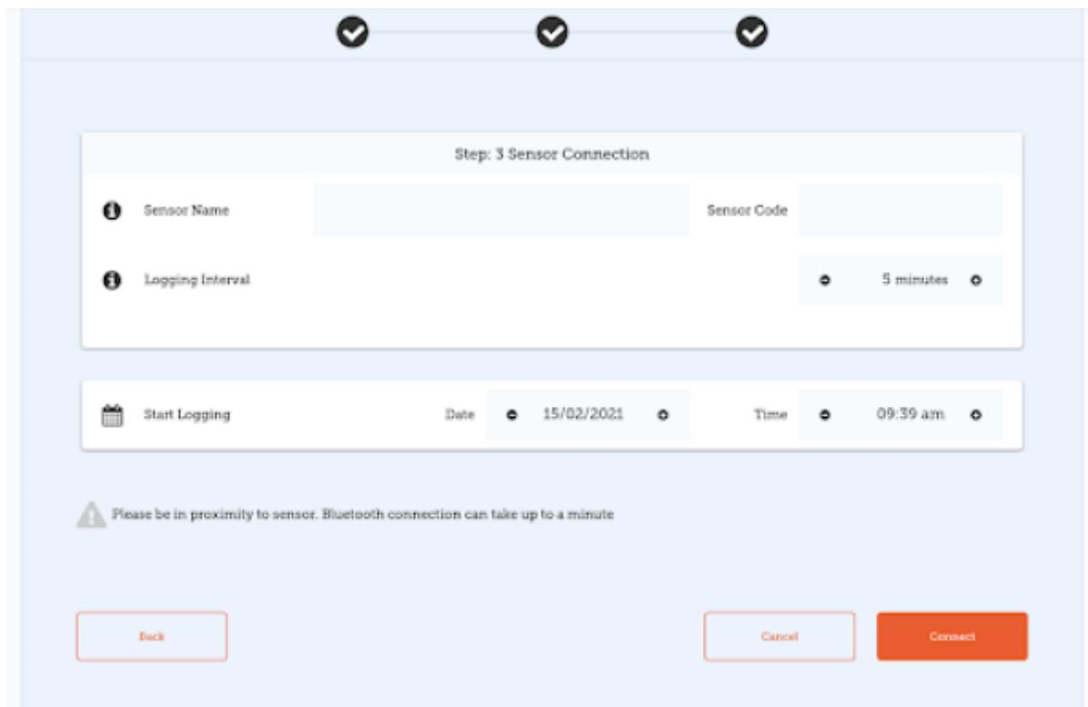
Tap **Connect** to complete sensor setup and add the sensor to mSupply mobile. This will return you to the mSupply mobile vaccine home screen and you will see the sensor has been added.
